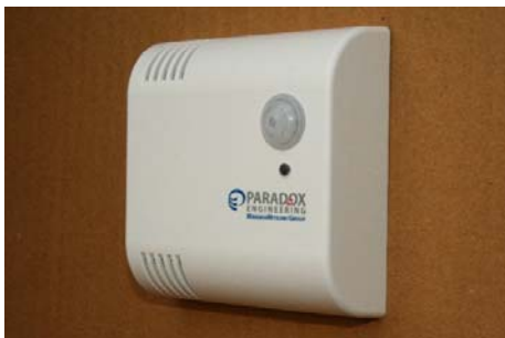
Figure 2: Indoor Smart Sensor Node (“PE_IoT_STONE_Multisensor” device) – Swiss Pilot
