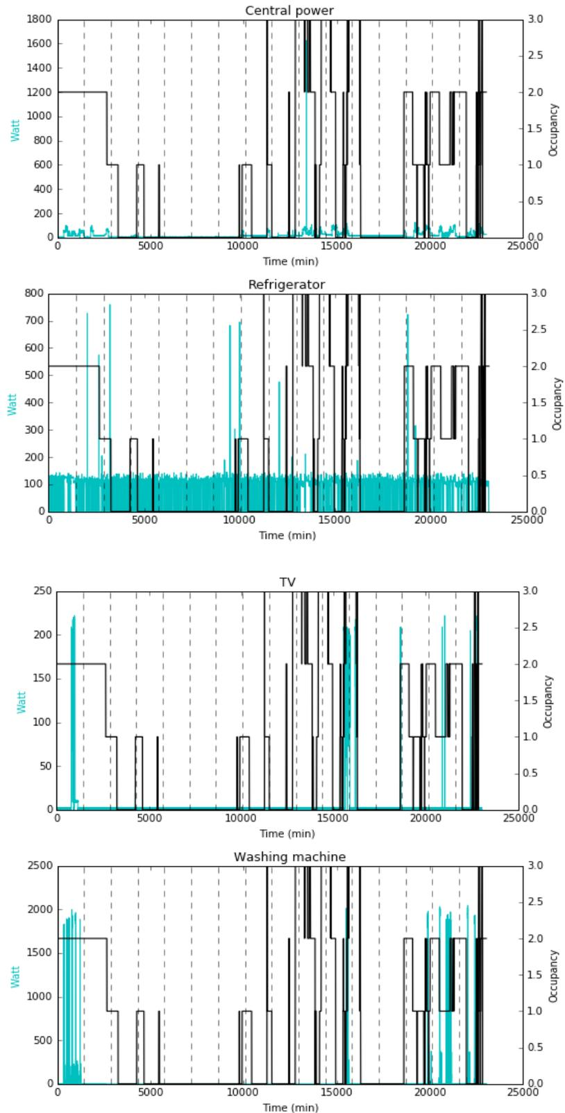
**Figure 7:** Energy consumption of electrical devices central power, refrigerator, TV and washing machine (cyan solid line - left axis) compare to occupancy (black solid line - right axis).
