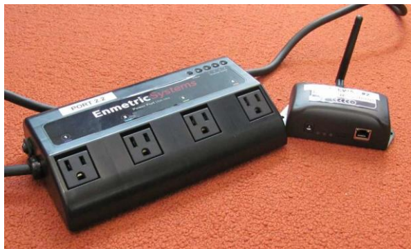
Figure 2: Enmetric plug monitoring system
